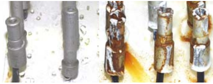
FIGURE 3. ASTM B117 Salt Spray Performance of end-fitting fasteners at 3000 hours using coating systems on left: Zinc plate with SM topcoated with chromate-containing heat-cured epoxy, and on right: Zinc plate with yellow chromate topcoated with same chromate-containing heat-cured epoxy.
