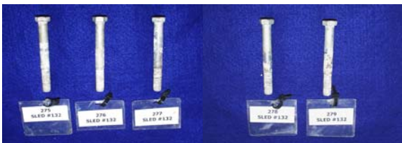
FIGURE 7. SM treated fasteners with an epoxy topcoat and no red rust at 60 cycles of Ford APG protocol testing.
