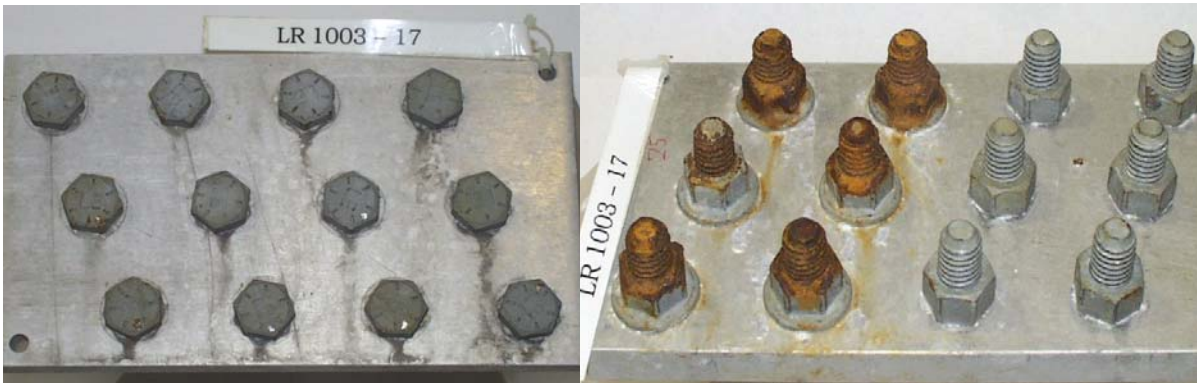
Group 17 – Product M – Heads (left) and Threads (right) at 180 cycles
