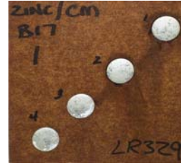
FIGURE 10. ASTM B117 Salt Spray 4000 Hour ASTM B117 Performance of the “bucked” rivets from Figure 9.
