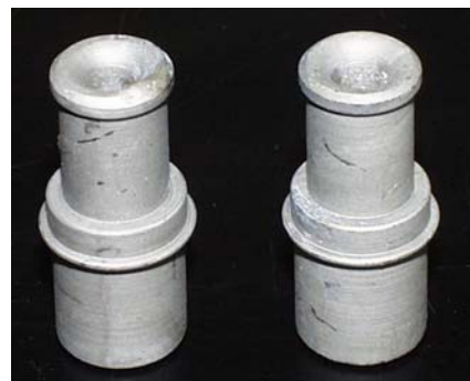
FIGURE 4. Brake Cable End Fittings zinc plated plus ESM and top coated with chromate free epoxy at 6552 hours ASTM B117 exposure.
