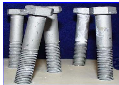
FIGURE 5. ASTM B117 Salt Spray Performance of Grade 8 bolts treated with ESM and top coated with chromate-free epoxy at 1000 hours.
