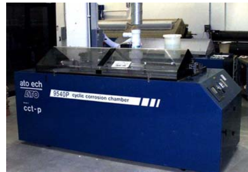
FIGURE 11. Test set up for GM-9540P cyclic testing of SM treated fasteners.
