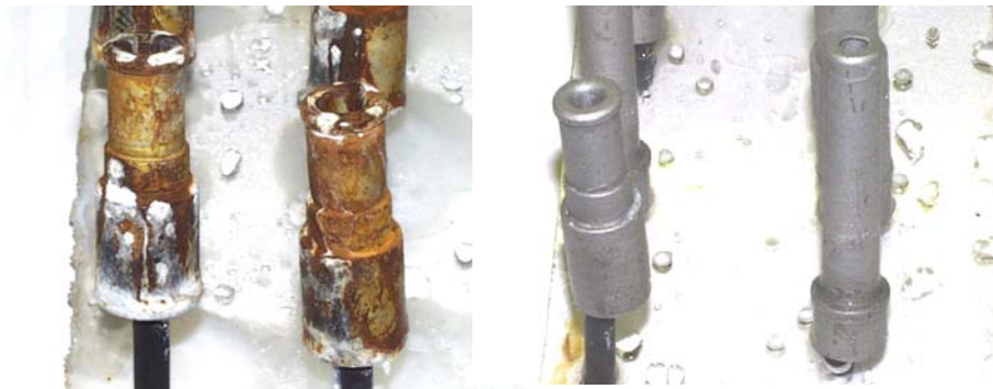
Conventional Zinc, Yellow Chromate, Heat Cured Epoxy topcoat After 3000hr ASTM B-117 Exposure
