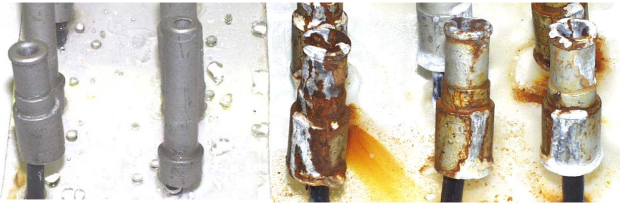
Figure 3: ASTM B117 Salt Spray Performance of end-fitting fasteners at 3000 hours using coating systems on left: Zinc plate with the mineral coating topcoated with chromate-containing heat-cured epoxy, and on right: Zinc plate with yellow chromate (Cr(VI)) topcoated with same chromate-containing heat-cured epoxy.
