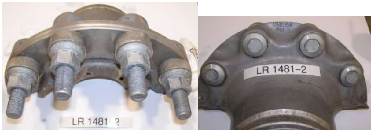
40 Cycles – Group 2 – Elisha 0251 General zinc corrosion (white rust) on threads and damaged areas of nut.
