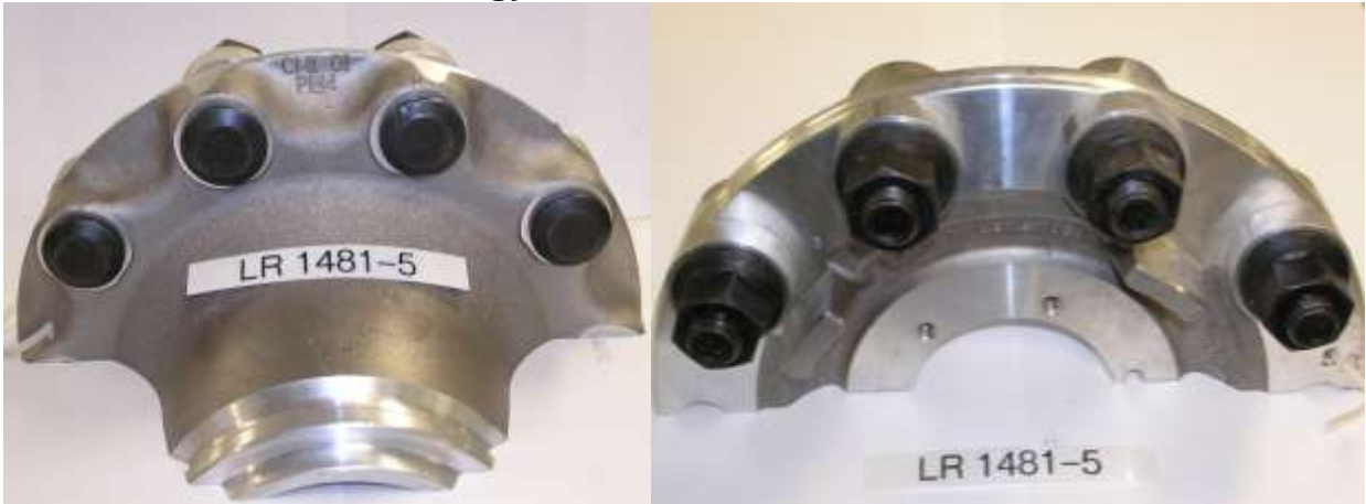
Pre-testing – Group 5 – Current Aluminum Wheel Manufacturer Coating
