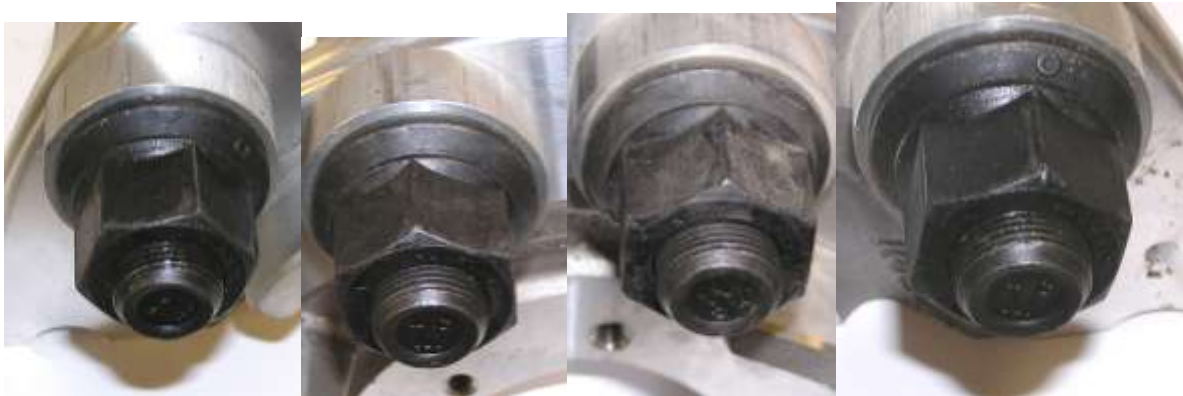
Pre-testing – Group 5 – Current Aluminum Wheel Manufacturer Coating Individual studs prior to corrosion testing.
