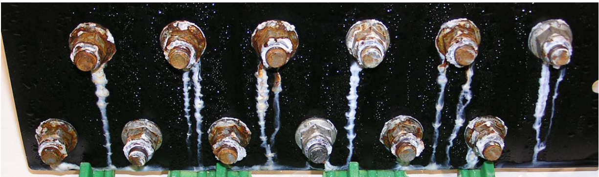
S440 Tri Cr3 – ASTM B-117 at 1008 hours
