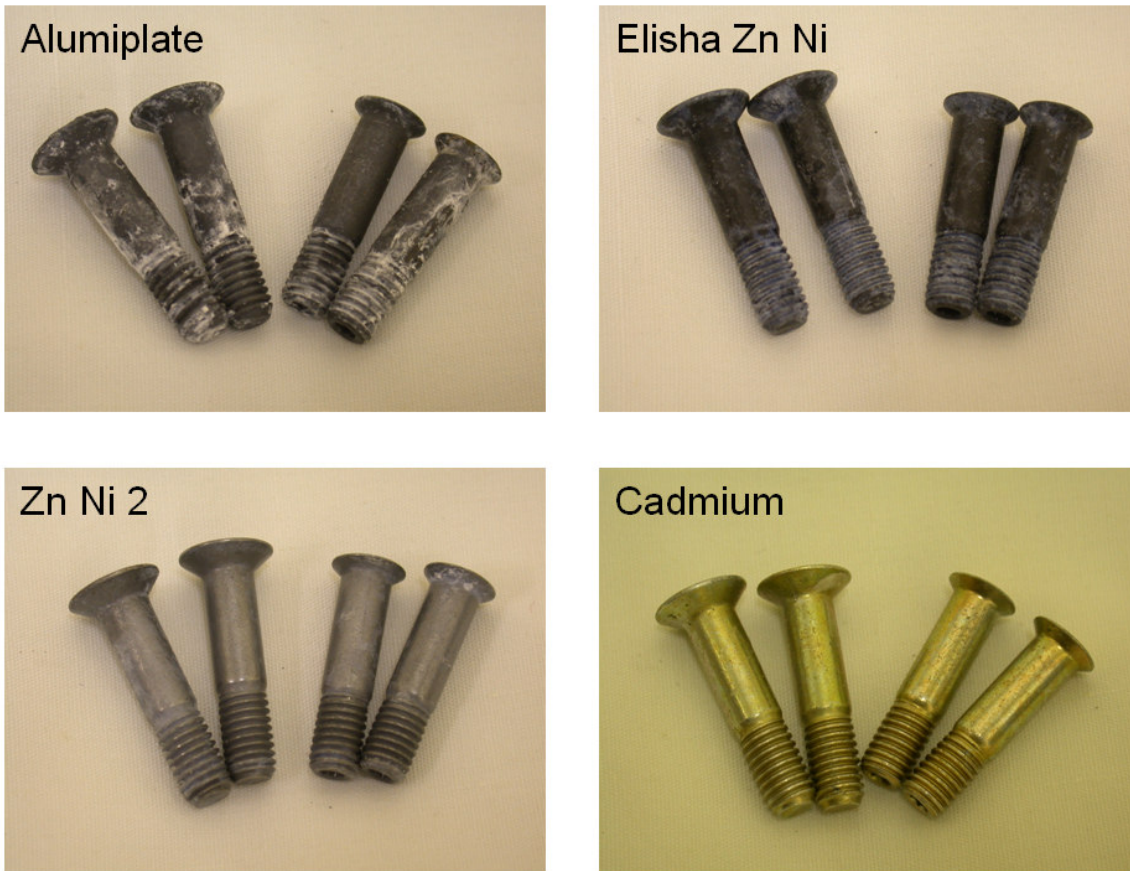
Figure 9 illustrates the appearance of the typical fasteners after 700 hours of salt spray test.
