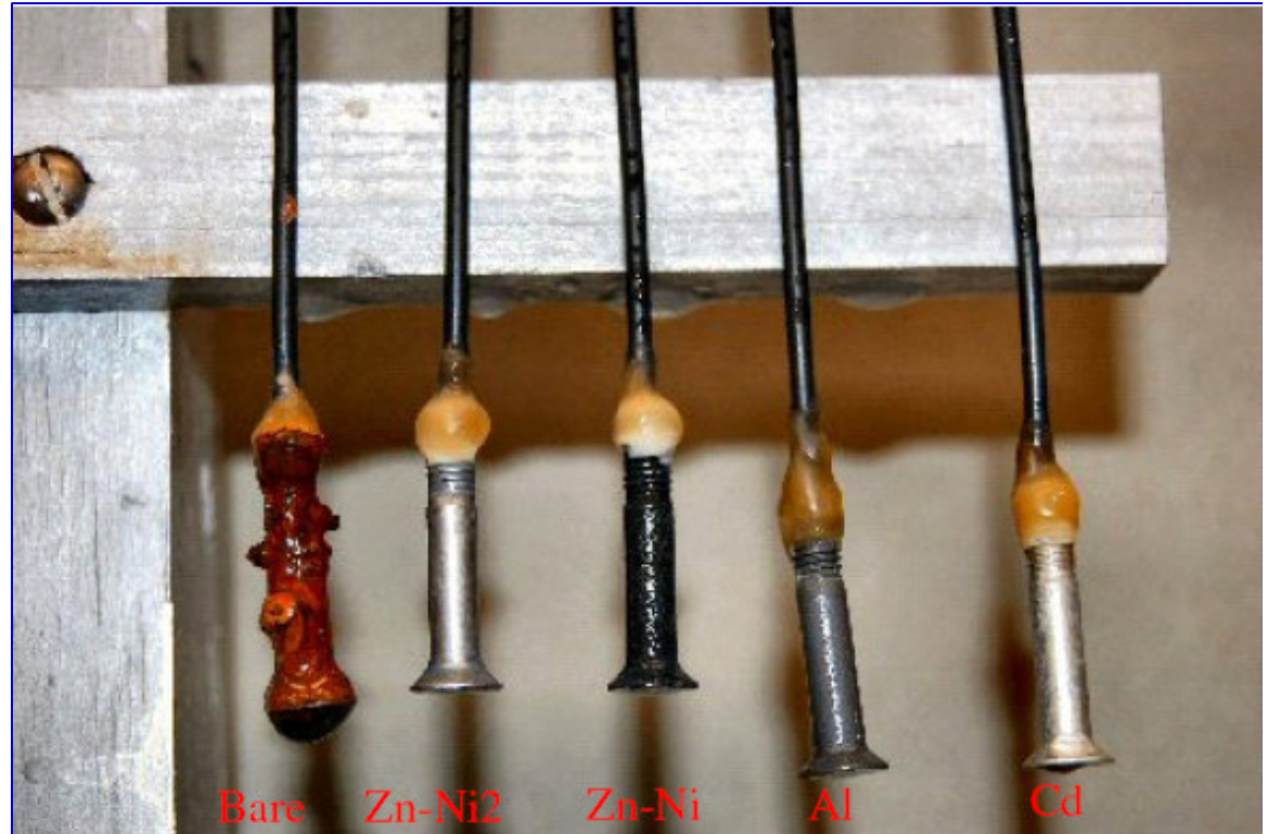
Corrosion potential measurement for salt spray
