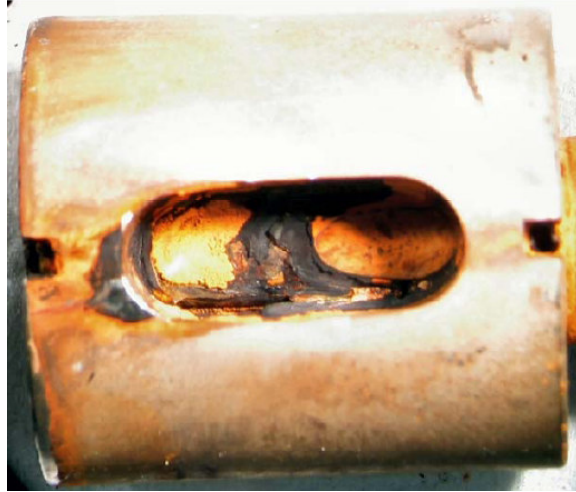
Figure 16 shows typical SCC Specimen in a steel collar, after 60 days test.
